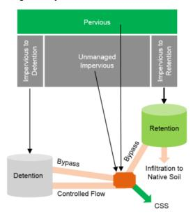
Figure 2. Stormwater pathways.<sup>18</sup>
