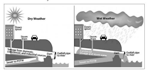
Figure 1. Combined Sewer Systems and Overflows.3
